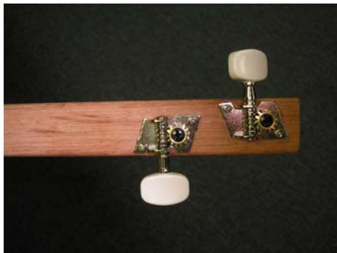
3. 1.5 inches from the tuning pegs, use a small hack saw to create a tiny groove to set the nut (1.5" piece of the 1/8<sup>th</sup> inch dowel) in place. The strings will run from the tuning pegs over this dowel and to the dowel that is the bridge. You don't want the strings to vibrate from the tuning pegs all the way to the bridge. A wooden nut and bridge will give a sweeter sound. Use white glue to secure the nut in place.
