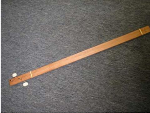
6. Drill two tiny holes side by side 3/4<sup>th</sup> of an inch past the bridge centered with 3/8<sup>th</sup>" between them. These are very tiny so you can then use these holes to screw in the tiny eyehooks. These eyehooks will hold the end of the strings.
