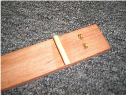
7. Drill two more tiny holes on the other side of the fingerboard in between the nut and the tuning pegs and screw in the tiny eyescrews. The strings will pass over the nut and go through the eyescrews before winding around the tuning pegs. The eyescrews should be screwed into the wood as far as they can go, and maybe even flattened down a bit. It is necessary for the eyescrews to pull the strings down onto the nut.
